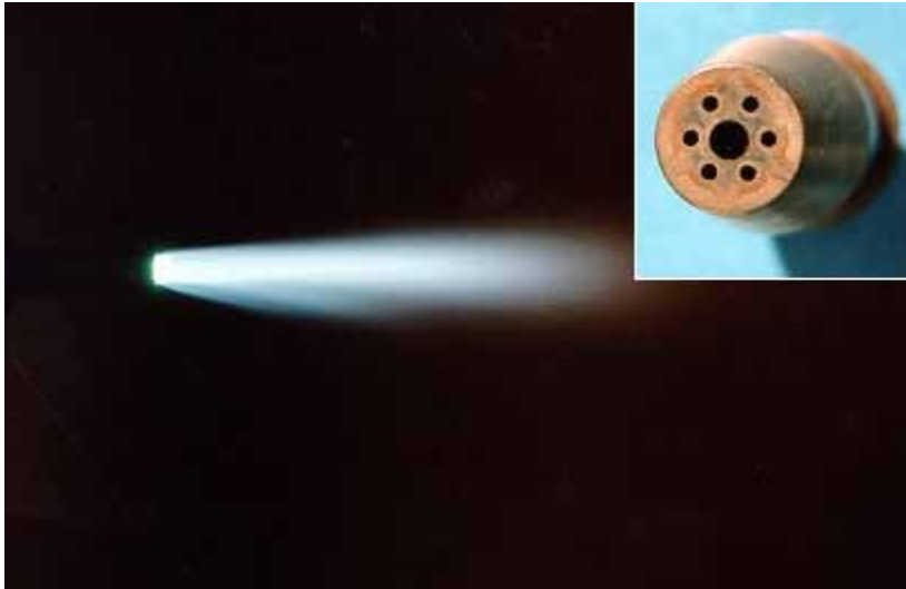
Fig.2. Oxyacetylene gas jet and nozzle design
