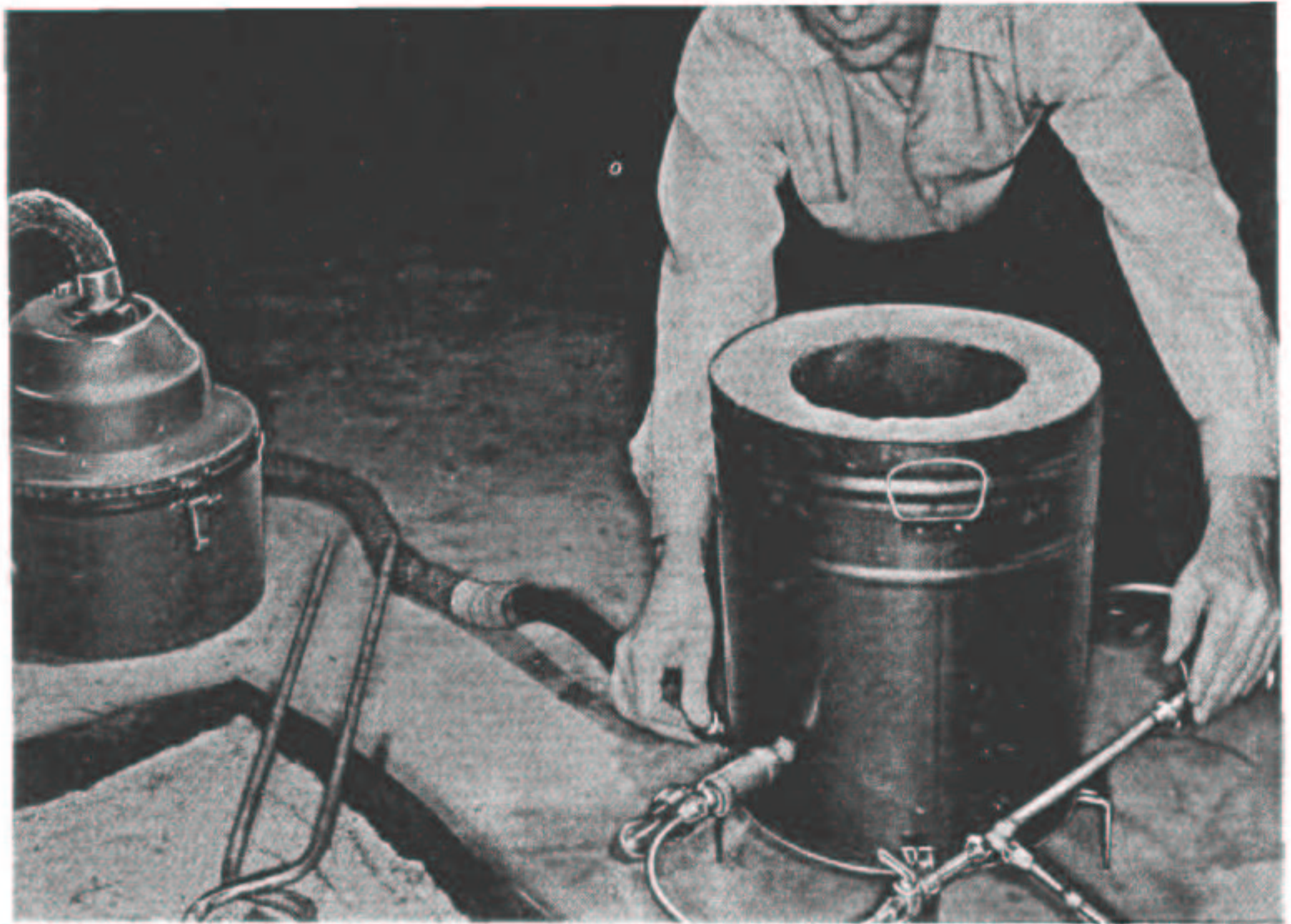
Here's the completed furnace set up ready for use. The burners have separate gas valves to provide precise adjustment of the flame. A single valve controls the air supply from the vacuum cleaner. Although not pictured, the molding flask should be placed near the furnace
