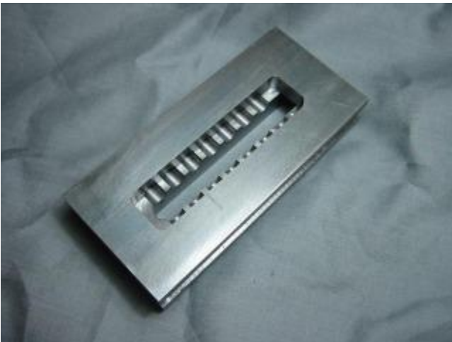
Cut path completely through from the bottom side.
