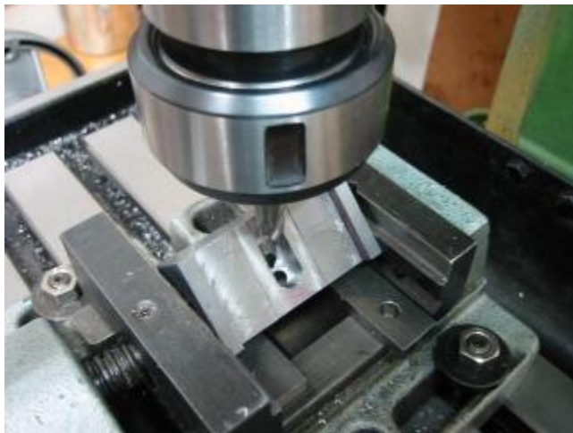
Machining a clearance for the tightening screw.
