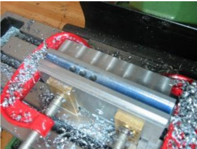
This deep hole drilling is a difficult yet a key process of the vise making. The depth is 50mm. All the holes must be straight and drilled at the accurate position.
