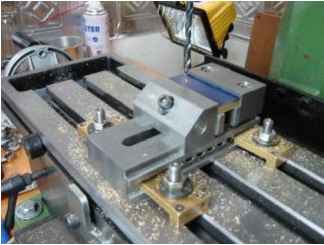
Machining the jaw plates with the vise temporary assembled
