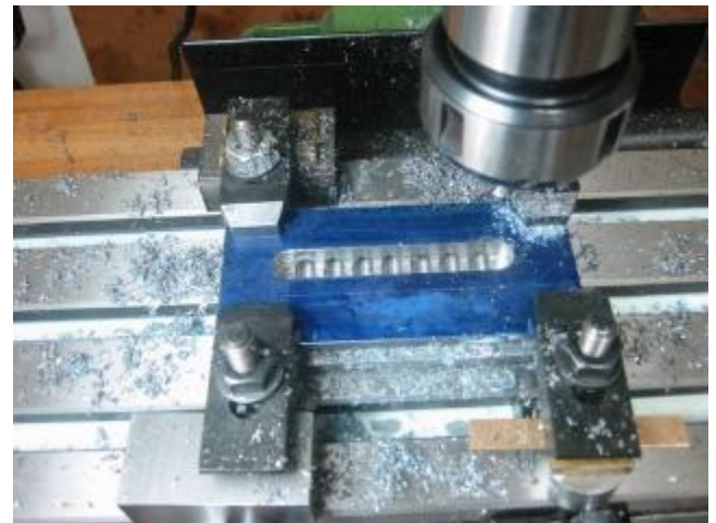
Slot cutting from the bottom side. The slot reaches to the one half of the hole diameter.
