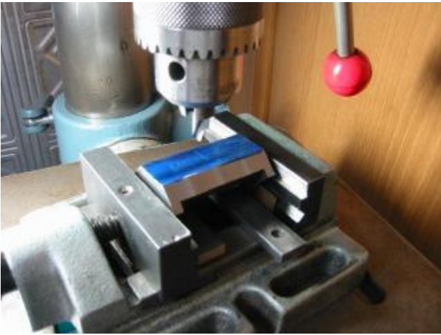
Drilling for the tightening screw.
