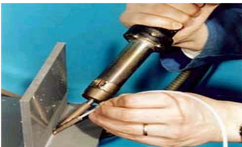
Hot Gas Welding
