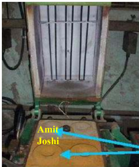
Shell parts on the heated pattern
