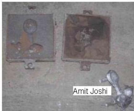
Casting removed from the boxes
