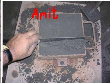
Box filled and excess sand removed
